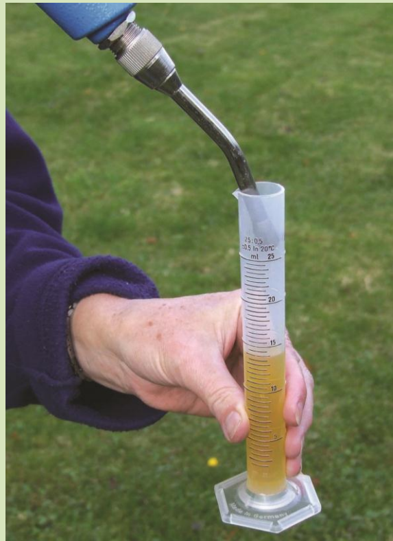
Checking dosing gun calibration
