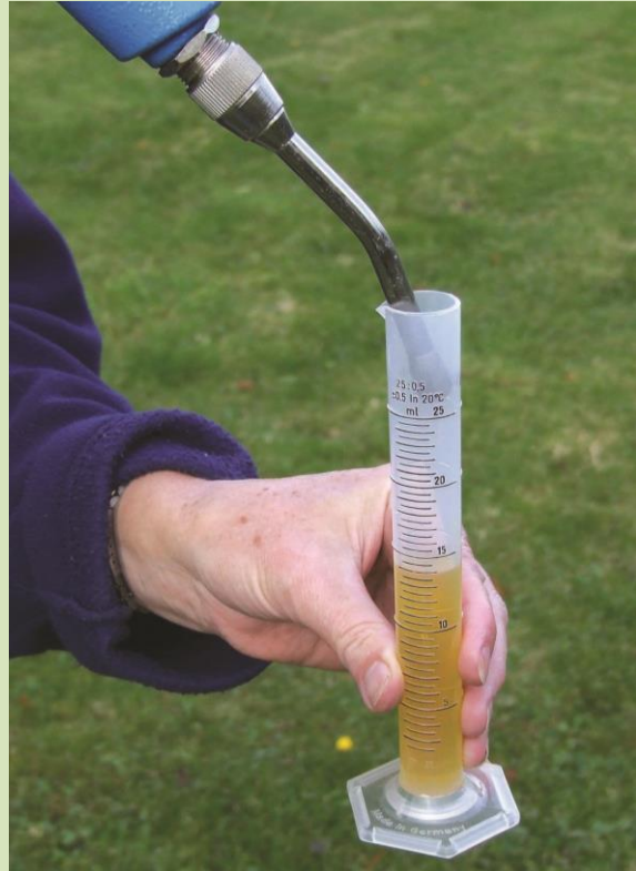
Checking dosing gun calibration
